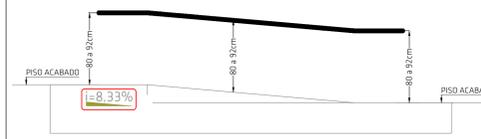
DETALHE DA RAMPA, CORRIMÃO EM PAREDE - IN 09 SEM ESCALA
