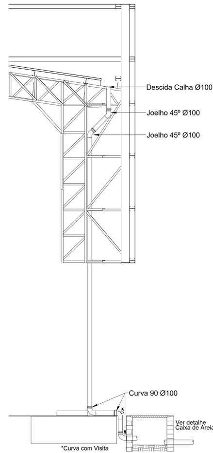
**6 DETALHE DESCIDA DAS AGUAS PLUVIAS.**
